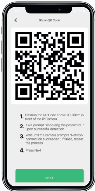
Position the shown QR code in front of the IP camera until it prompts " Receiving the password ". Wait until the network connection succeeded Tap NEXT
